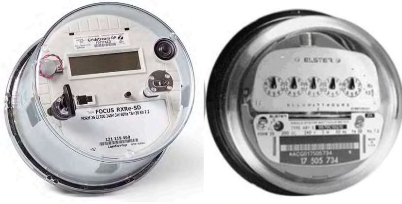
Figure 2 A modern, advanced electric meter (left) and an older, analog meter (right)
