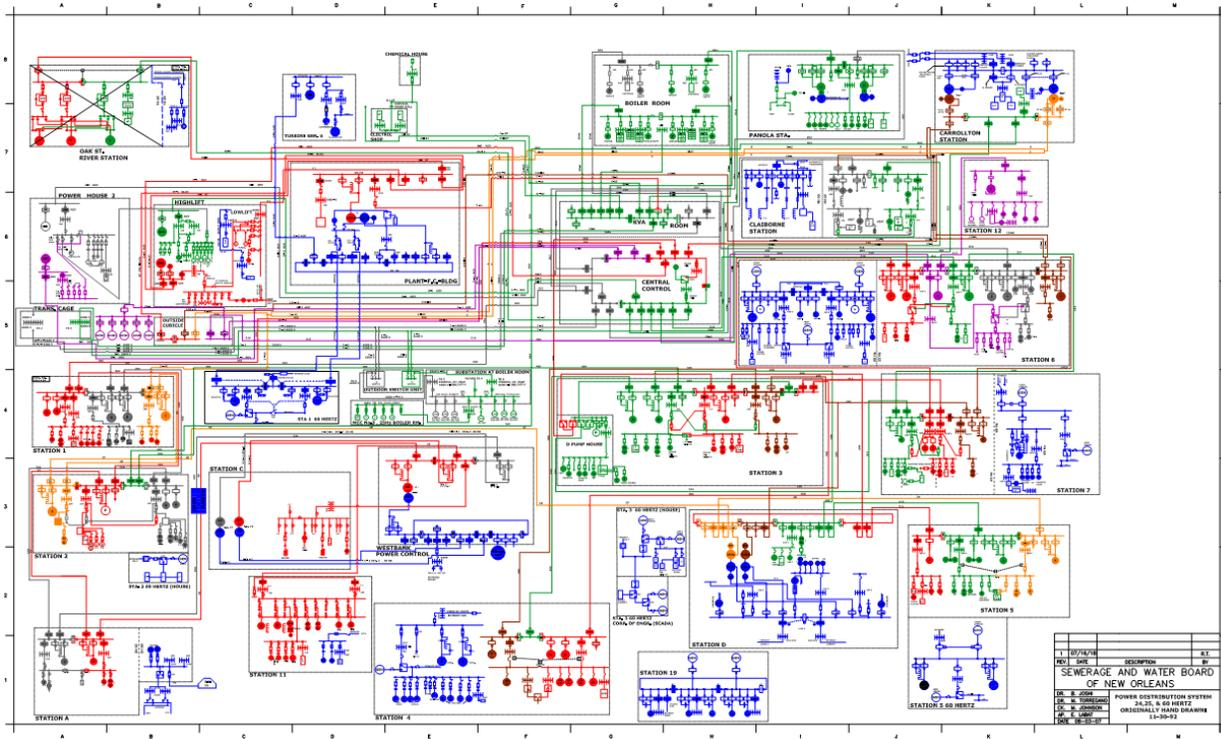
**Figure 2-3. SWBNO 24, 25 and 60 Hz Power Distribution Network**
